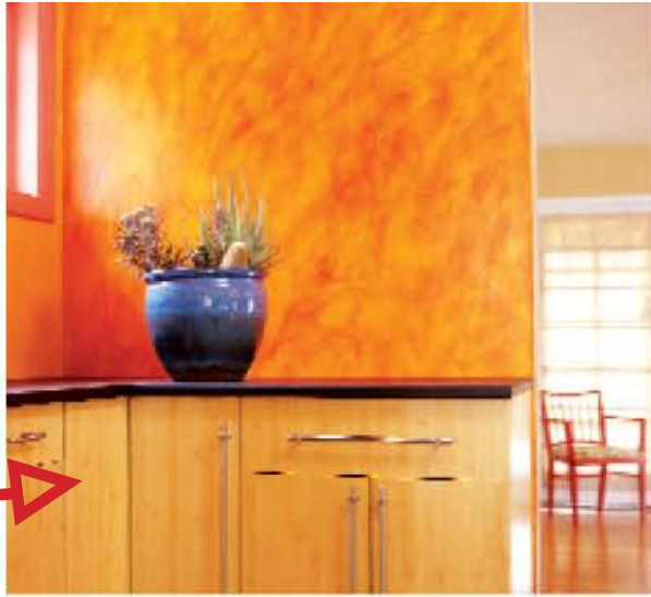
▲ Bamboo makes an excellent choice for cabinets; it's strong, flexible, and offers a natural finish.
